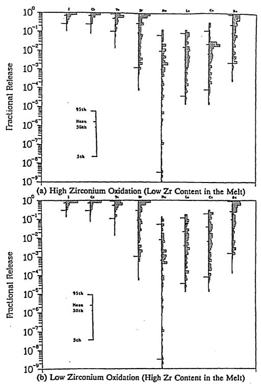
Uncertainty Distributions for Total Releases Into Containment BWR, Low Pressure Fast Station Blackout, Limestone Concrete, Dry Pedestal, Low Drywell Temperature, FPART = 1.
